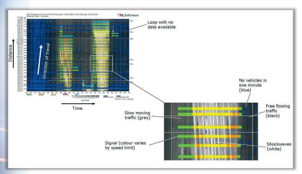
The live and historic information provided by MotorGraph allows licensed users to assess and track operational performance of control systems on motorways, monitor live and historic traffic patterns, optimise traffic control systems and identify sources and causes of congestion.
